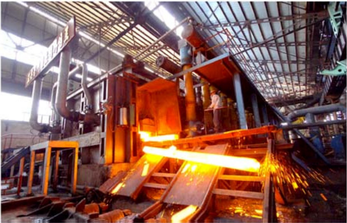
A medium-sized heating oven for rolling based on the high-temperature air combustion technology at the Chollima Steel Complex.
