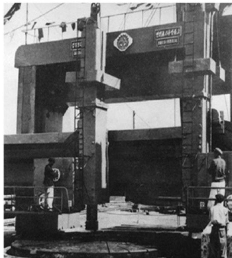
Workers at the Ryongsong Machine Plant completing the assembling of an 8-metre turning lathe
